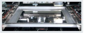
Automatic push-up pin exchange function (Option) Automatically places push-up pins to support the board during the print process. The magnetic pins are automatically placed at optimal positions matching the shape and pattern of the circuit board, avoiding pre-placed components. This achieves stable and repeatable printing support for every program.
